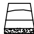
HALF BLOCK (SHOULD BE CAST WITHOUT TONGUE TO AVOID CUTTING IN THE FIELD)
